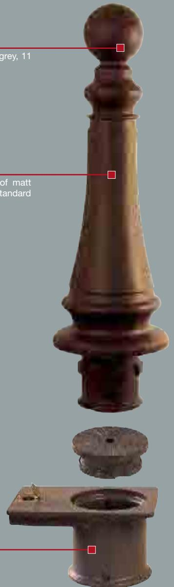
The FIXATOR system is an URBACO patent, and enables manual release of a removable bollard. After having removed it, the cover frees the passage way by covering the hole on the ground. Fixator is secured to the ground using cement. It's collision resistance depends on the quality and dimensions of the anchoring
